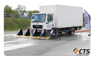
Blockers | Retractable Manufacturer:TISO Production Ltd Standard Tested To: IWA 14-1:2013 Performance rating: V/7200[N2A]/48/90/25.4
