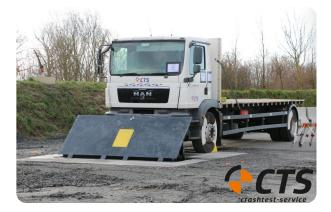
Blockers | Retractable Manufacturer:TISO Production Ltd Standard Tested To: IWA 14-1:2013 Performance rating: V/7200[N3C]/80/90:0
