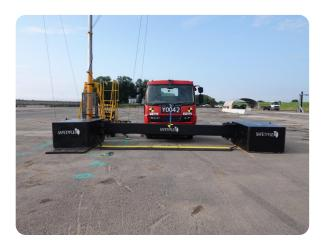
Gates | Swing Manufacturer:Safetyflex Barriers Standard Tested To: IWA 14-1:2013 Performance rating: V/7200[N2A]/64/90:6.1
