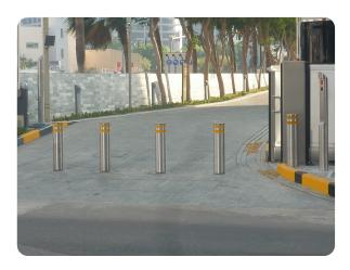
Bollards | Retractable Manufacturer:ATG Access Standard Tested To: PAS 68:2007 Performance rating: V/7500[N2]/48/90:0/0.0
