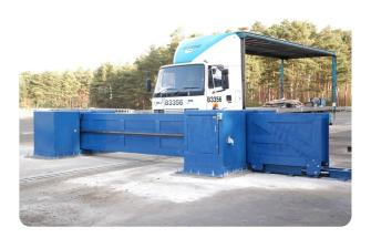
Gates | Sliding Manufacturer:Barkers Fencing Standard Tested To: Development test meeting PAS 68:2005 Performance rating: V/7500[N3]/80/90:0/0.0
