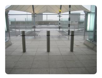
Bollards | Static Manufacturer:ATG Access Standard Tested To: PAS 68:2007 Performance rating: V/7500[N2]/48/90:6.9/0.0
