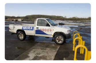
Bollards | Static Manufacturer:Safetyflex Barriers Standard Tested To: PAS 68:2007 Performance rating: V/2500[N1G]/64/90:0.9/0.0
