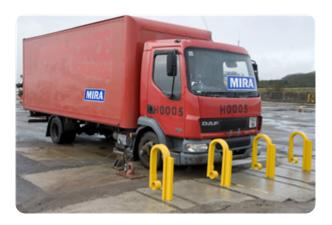
Bollards | Static Manufacturer:Safetyflex Barriers Standard Tested To: PAS 68:2007 Performance rating: V/7500[N2]/48/90:3.7/5.2
