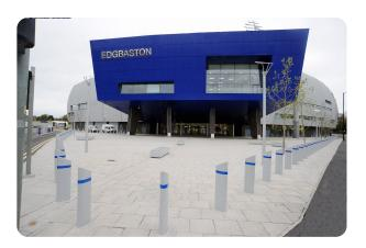
Bollards | Static Manufacturer:Safetyflex Barriers Standard Tested To: PAS 68:2007 Performance rating: V/7500[N2]/48/90:0/0.0
