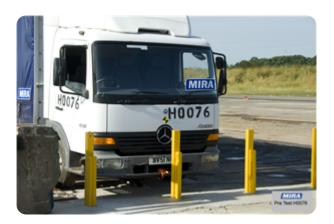
Bollards | Static Manufacturer:Safetyflex Barriers Standard Tested To: PAS 68:2007 Performance rating: V/7500[N2]/48/90:1.2/0.0
