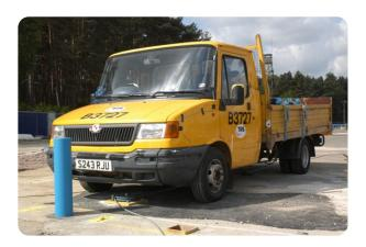
Bollards | Static Manufacturer:Leda-Vannaclip Standard Tested To: PAS 68:2007 Performance rating: V/3500[N1]/48/90:0/0.0
