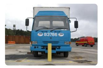
Bollards | Static Manufacturer:Leda-Vannaclip Standard Tested To: PAS 68:2007 Performance rating: V/7500[N2]/32/90:0/0.0
