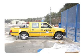
Perimeter Barriers | Pedestrian Manufacturer:Barkers Fencing Standard Tested To: PAS 68:2007 Performance rating: V/2500[N1G]/48/90:0/0.0
