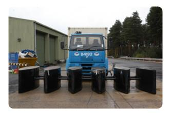
Perimeter Barriers | Modular Manufacturer:Systra Ltd Standard Tested To: PAS 68:2007 Performance rating: V/7500[N3]/64/90:5.4/0.0
