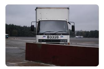
Perimeter Barriers | Vehicle Manufacturer:Systra Ltd Standard Tested To: Development test meeting PAS 68:2005 Performance rating: V/7500[N2]/80/45:0/15.0
