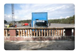
Perimeter Barriers | Vehicle Manufacturer:Systra Ltd Standard Tested To: Development test meeting PAS 68:2005 Performance rating: V/7500[N2]/48/90:0/7.5
