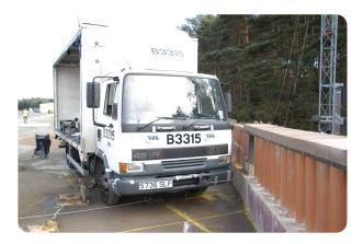
Perimeter Barriers | Vehicle Manufacturer:Systra Ltd Standard Tested To: Development test meeting PAS 68:2005 Performance rating: V/7500[N2]/80/30:0/0.0
