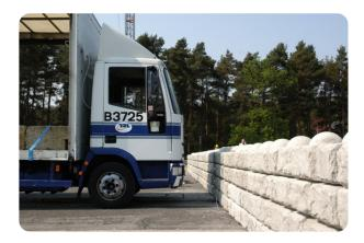
Perimeter Barriers | Vehicle **Manufacturer:**Marshalls Civils and Drainage **Standard Tested To:** PAS 68:2007 **Performance rating:** V/7500[N2]/48/90:1.6/0.0
