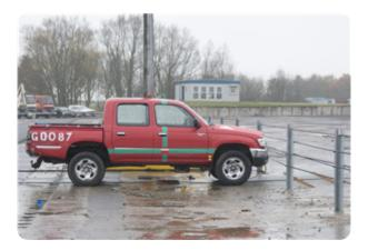
Perimeter Barriers | Vehicle Manufacturer:ATG Access Standard Tested To: PAS 68:2007 Performance rating: V/2500[N1G]/48/90:1.6/0.0
