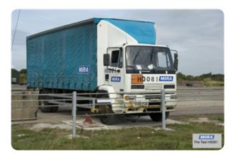
Perimeter Barriers | Vehicle Manufacturer:Jacksons Fencing Ltd Standard Tested To: PAS 68:2007 Performance rating: V/7500[N3]/80/90:12.1/0.0
