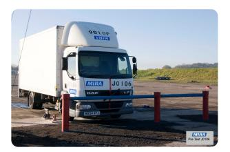
Perimeter Barriers | Vehicle **Manufacturer:**Eagle Automation Systems Limited **Standard Tested To:** PAS 68:2010 **Performance rating:** V/7500[N2]/48/90:1.5/0.0
