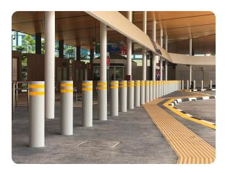
Bollards | Static Manufacturer:ATG Access Standard Tested To: PAS 68:2010 Performance rating: V/7500[N2]/48/90:0/0.0
