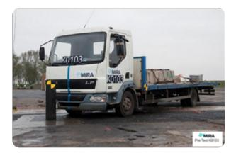
Bollards | Retractable **Manufacturer:**Security Solutions Northern Ltd **Standard Tested To:** PAS 68:2010 **Performance rating:** V/7500[N2]/48/45:1.1/0.0
