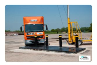
Bollards | Sliding Manufacturer:Heald Ltd Standard Tested To: PAS 68:2010 Performance rating: V/7500[N2]/48/45:0.8/0.0
