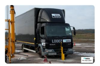
Bollards | Retractable Manufacturer:Safetyflex Barriers Standard Tested To: PAS 68:2010 Performance rating: V/7500[N2]/48/45:2.6/2.2
