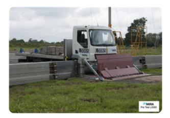
Blockers | Retractable **Manufacturer:**Multiple manufacturers (see specification) **Standard Tested To:** PAS 68:2010 **Performance rating:** V/7500[N2]/48/90:1.5/0.0
