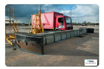
Perimeter Barriers | Modular Manufacturer:Highway Care Ltd Standard Tested To: IWA 14-1:2013 Performance rating: V/7200[N2A]/48/90:5.5
