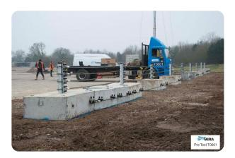
Perimeter Barriers | Vehicle Manufacturer:Safetyflex Barriers Standard Tested To: IWA 14-1:2013 Performance rating: V/7200[N3C]/80/90:6.8
