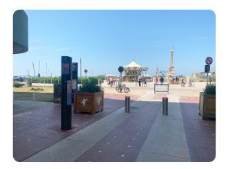
Bollards | Retractable Manufacturer:CAME Urbaco Standard Tested To: IWA 14-1:2013 Performance rating: V/2500[N1G]/48/90:0.6
