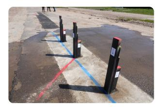
Bollards | Static Manufacturer:Safetyflex Barriers Standard Tested To: IWA 14-1:2013 Performance rating: V/7200[N2A]/64/45:3.3
