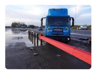
Perimeter Barriers | Vehicle Manufacturer:ATG Access Standard Tested To: IWA 14-1:2013 Performance rating: V/7200[N2A]/48/30:0.2
