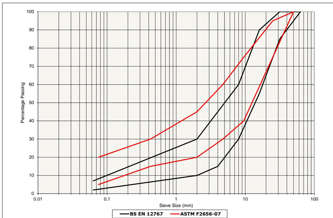
Figure 1: Comparison of grading envelopes
