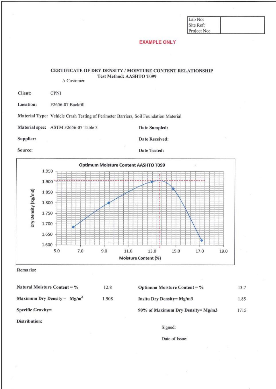
**Figure 8: Example Dry Density / Optimum Moisture Content Report**
