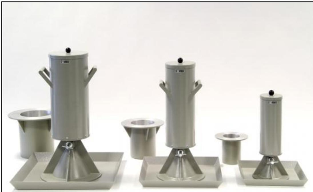
Figure 3: BS 1377 Part 9 Sand Replacement Equipment
