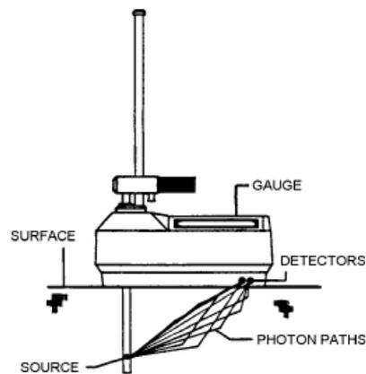
Figure 5b: Direct Transmission mode
