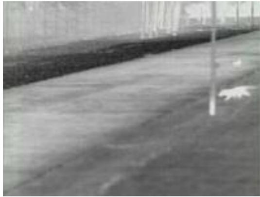
Figure 2: Pre-alarm video still of a false alarm cause (fox), captured with thermal imager
