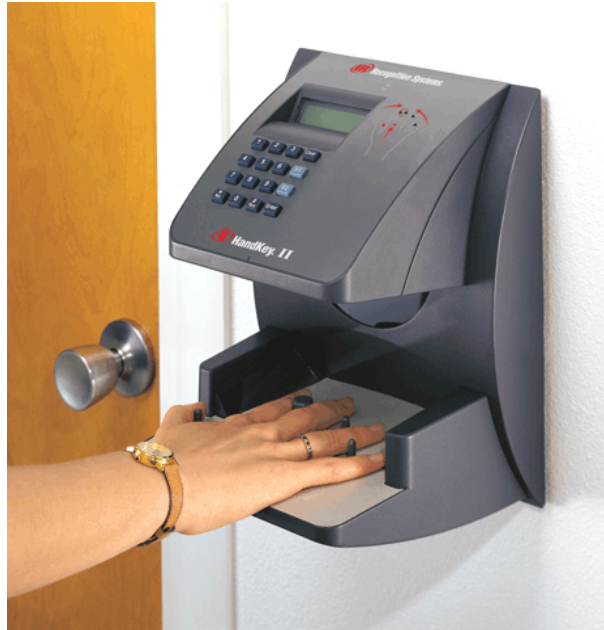
Figure 2: Hand geometry device (used with permission of Ingersoll Rand Security Technologies)
