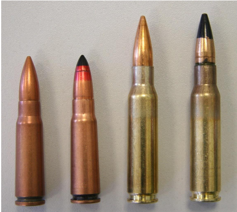
Fig2: AK-47 7.62x39 and NATO 7.62x51 ammunition – ( L to R: PS ball round, BZ API round, NATO ball round, NATO AP round)
