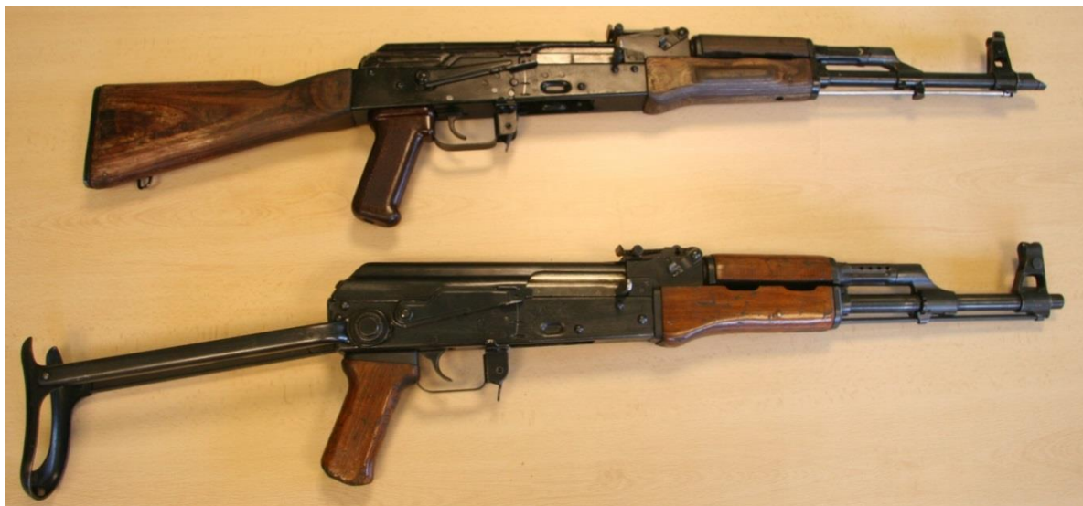
Fig.1: AK-47 Assault rifles – (T to B: AK-47 and AKM)
