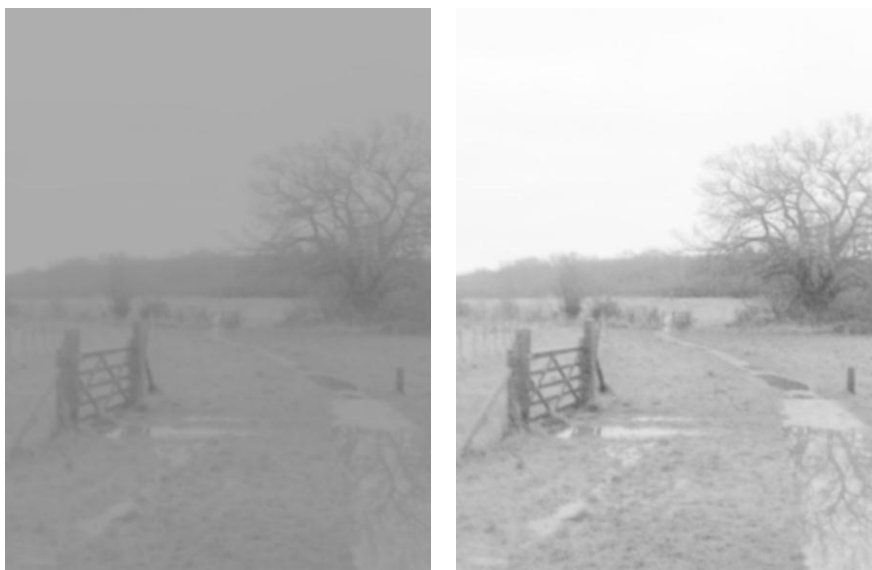
Figure 4: How image processing can increase contrast in a thermal image to provide greater detail.
