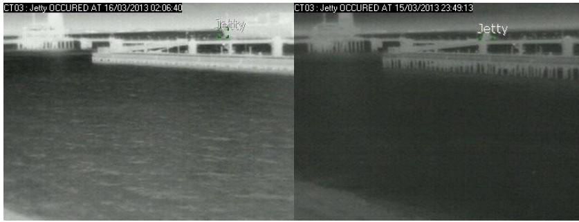
Figure 2: Two images of the same scene (mooring and jetty viewed over water). On the left an image under good conditions, on the right reduced thermal information.
