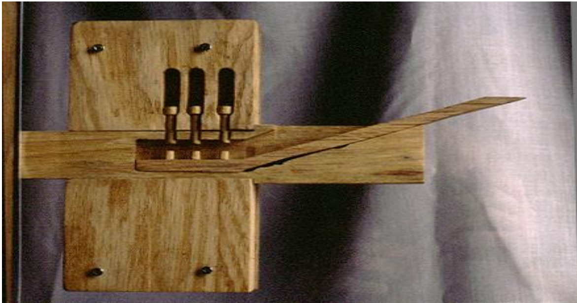
Illustration 1: Egyptian wood pin-tumbler lock
